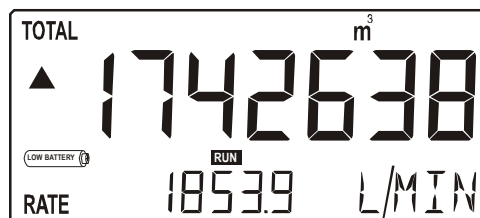
Fig. 4: Example of low-battery alarm.
